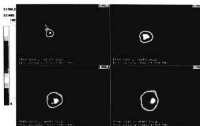
Figure 9. The first 150 msec of diastole in the Milwaukee Heart ventricle showing the wash-in of the ^{99m}\text{Tc} bolus. There is total dispersal of the bolus without any evidence of recirculating flow.
