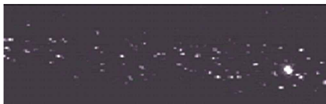
Figure 4 | Increased field of view limitations. Due to decreased magnification and resolution of the sample caused by an increase in the width of the field of view (FOV), a balance must be achieved between the number of particles that can be viewed at each frame and the precise visualization of individual particles.
